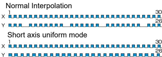
In 2-axis linear interpolation driving, axis which drives longer (long axis) keeps to output pulses continuously. Meanwhile, axis which drives shorter (short axis) sometimes outputs pulses by interpolation calculation result and sometimes does not. MCX512 has short axis pulse uniform function. For short axis, drive pulses are output making pulse interval uniform as much as possible.
