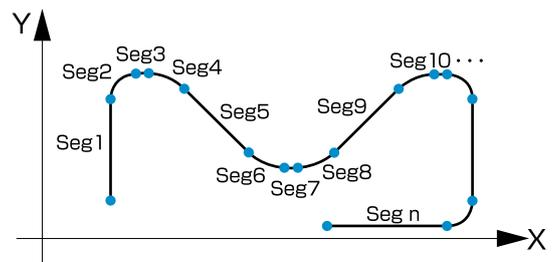
8 steps pre-buffer registers are equipped to execute high speed continuous interpolation driving. Continuous interpolation can be executed if there is short segment like Seg.3 in the above figure, when average drive time of 8 segments is longer than position data set time of next segment.
