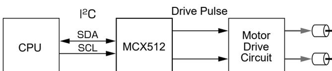
In addition to 8/16bit data bus, MCX512 can connect to the master CPU with I<sup>2</sup>C serial interface bus. Max 8pcs of MCX512 can be connected to one interface bus.
