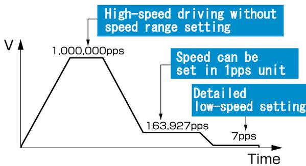
MCX512 has no speed multiple, speed can be set 1pps unit. This IC can change the speed directly from low speed, 1pps, 2pps to high speed pulse like 1Mpps during driving.
