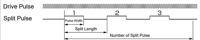
This is the function which outputs split pulse during driving. Synchronizing an axis's movement, various kinds of actions can be performed in specified intervals. By combining the split pulse output and the synchronous action, start/stop split pulse from a specified position and split length and pulse width can be changed by external signal input.
