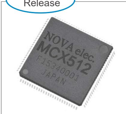
MCX512 is 2-axis Motion Control IC which connects to CPU with 8/16-bit or I<sup>2</sup>C serial interface bus and can control either a stepper motor driver or pulse type servo driver for position and speed.
