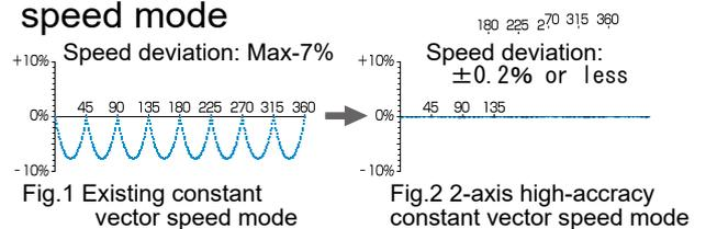
Besides existing constant vector speed mode, MCX512 has 2-axis high accuracy constant vector speed mode which is significantly improved constant vector speed mode. Short axis pulse uniform mode and 2-axis high accuracy constant vector speed mode are used together in 2-axis linear interpolation and circular interpolation, speed deviation of vector speed is ±0.2% or less. Drastic accuracy improvement of speed in interpolation driving is expected.
